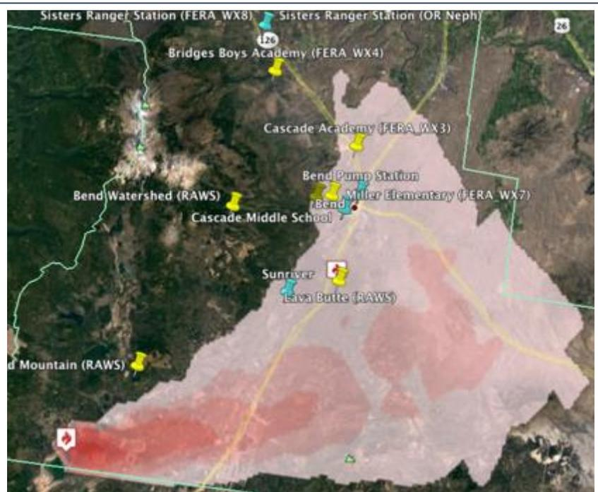
**Figure 3.** Meteorological and smoke measurement locations in the town of Bend, Oregon and south of town and the burn locations for the May 4-6, 2015 smoke intrusion period. The red contours are the near-surface 1-hr  $PM_{2.5}$  concentrations predicted by the BlueSky smoke modeling framework May 4, 2015 at 1400 PDT.
