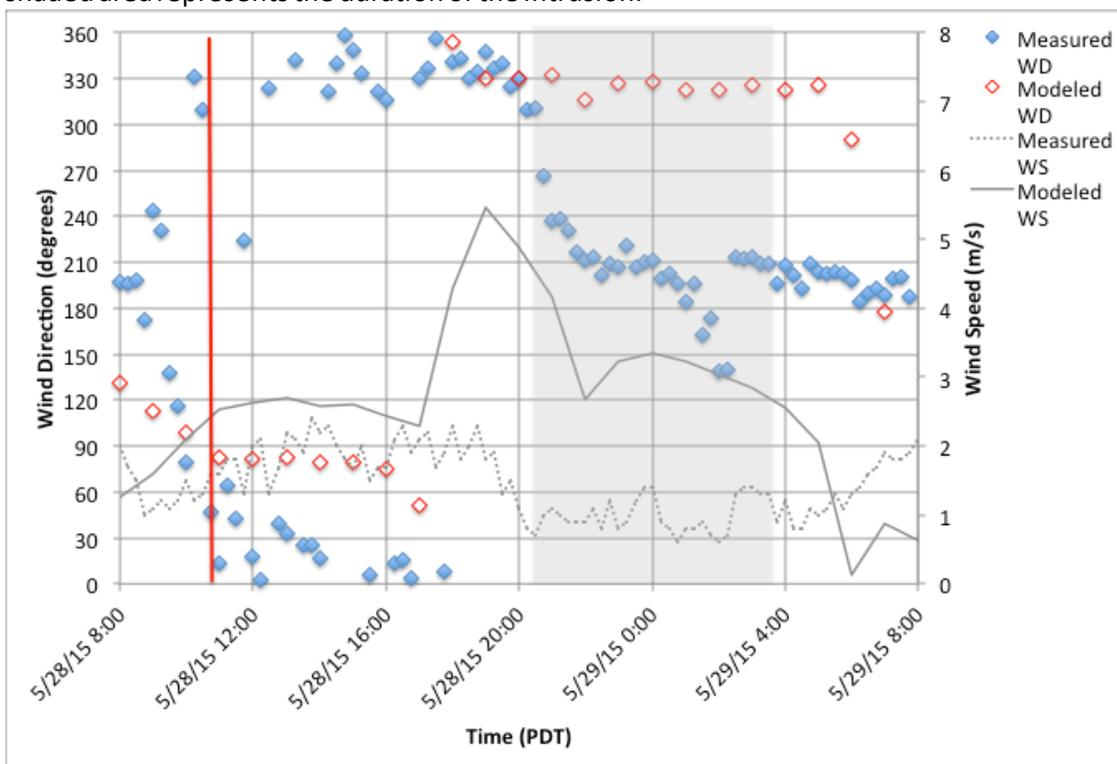
**Figure 10.** Measured and modeled wind speed and direction at Cascade Middle School, May 28, 2015 Rx burn. The red line designates ignition time, and the shaded area represents the duration of the intrusion
