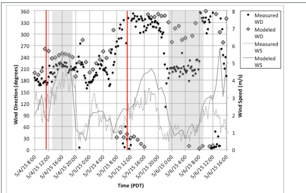
**Figure 6.** Measured and modeled wind direction and wind speed at Cascade Middle School for May 4-6, 2015. Red lines indicate burn ignition times and gray-shaded areas indicate the smoke intrusion periods into Bend, Oregon.
